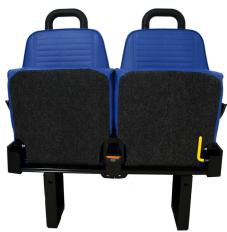
Available as a single or double passenger assembly, the EconoFlip has been designed with an easy to install, innovative connecting system allowing single units to be efficiently ganged together over any wheel well for multiple passenger, perimeter seating applications. The infinitely adjustable legs provide flexibility and reduced installation time.
